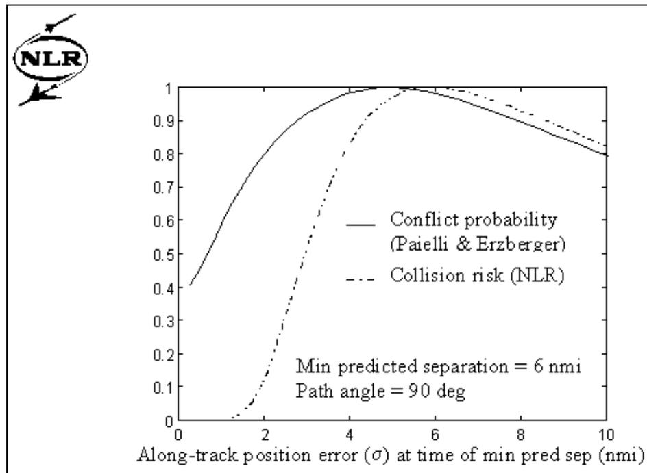
*Example :* Path angle is 90 degrees, minimum predicted separation is 6 nmi and the along-track rms position error at time of minimum predicted separation is varied (by changing the starting positions of both a/c) from 0.25 to 10 nmi.
