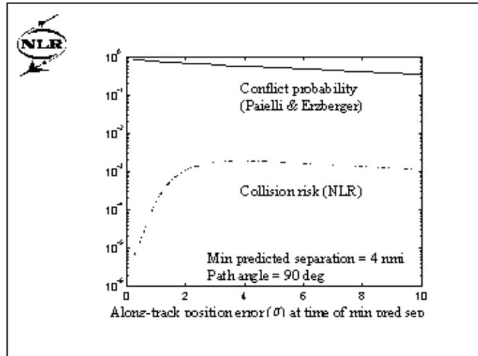
*Example :* Path angle is 90 degrees, minimum predicted separation is 4 nmi and the along-track rms position error at time of minimum predicted separation is varied (by changing the starting positions of both a/c) from 0.25 to 10 nmi.
