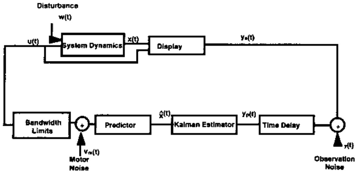
Figure1. Optimal Control Model. In this model the human operator is assumed to observe a display of system state and to compare that display to an internal model of the system, represented as a Kalman estimator and predictor. The operator then chooses an action that will offset any observed error between current and desired system state and acts through his neuromotor processes, which include a noise and bandwidth limit, to effect the control.
