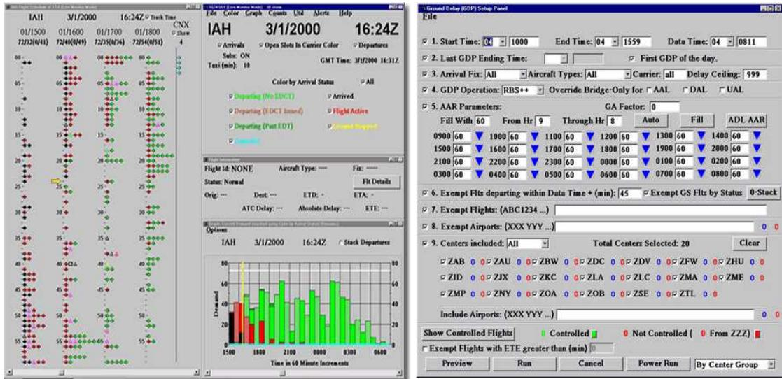
Figure 7: Flight Schedule Monitor predicts traffic flow by using shared information between ATM and AOC. [23]
