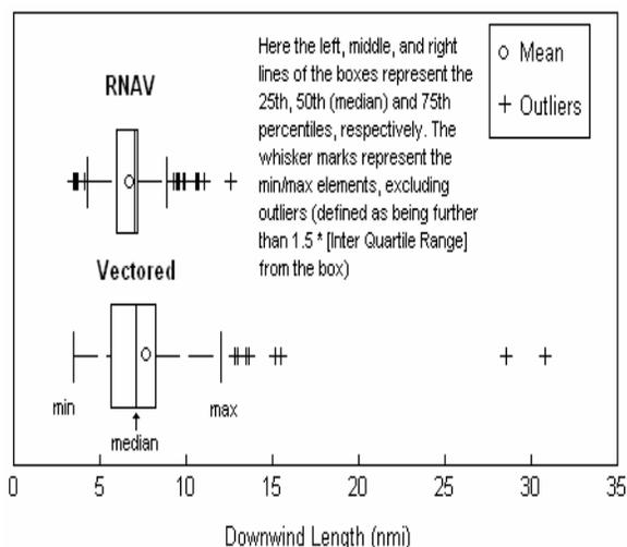
**Figure 6. Box and Whisker Plot of Downwind Lengths**
