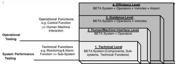
Figure 4: BETA Levels of Testing
