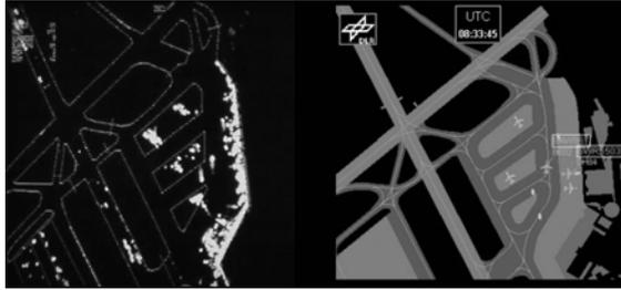
Figure 1: ASDE vs. A-SMGCS Controller HMI
